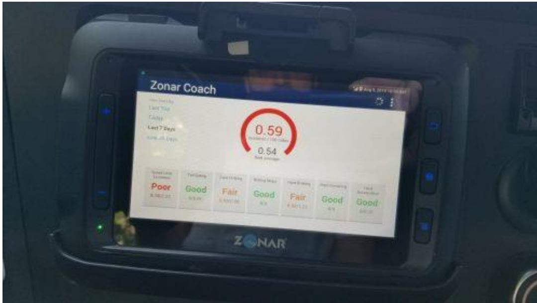
P&B Transport is using Zonar Coach, a camera-based driver safety and performance management system, that gives drivers feedback on a variety of metrics.
