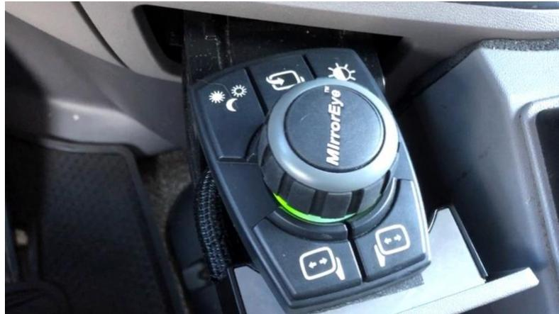
A control module allows drivers to pan the field of view slightly left or right, retract the camera wings, and adjust the brightness of image in the monitor to suit their taste.
