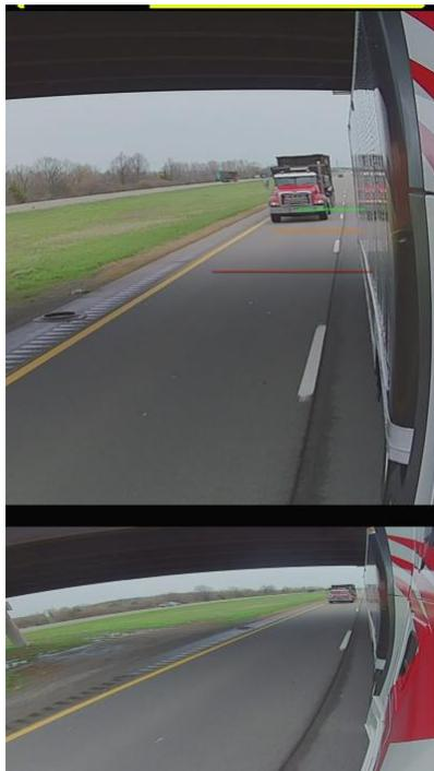
to glance at the monitor occasionally to verify or compare what I was seeing in the monitor to what I saw in the mirror. Since Stoneridge is presently the only supplier with a U.S. FMCSA exemption allowing it to operate trucks without conventional external glass mirrors, ignoring the A-pillar-mounted monitors wasn't an option on this test drive. They were all I had.
