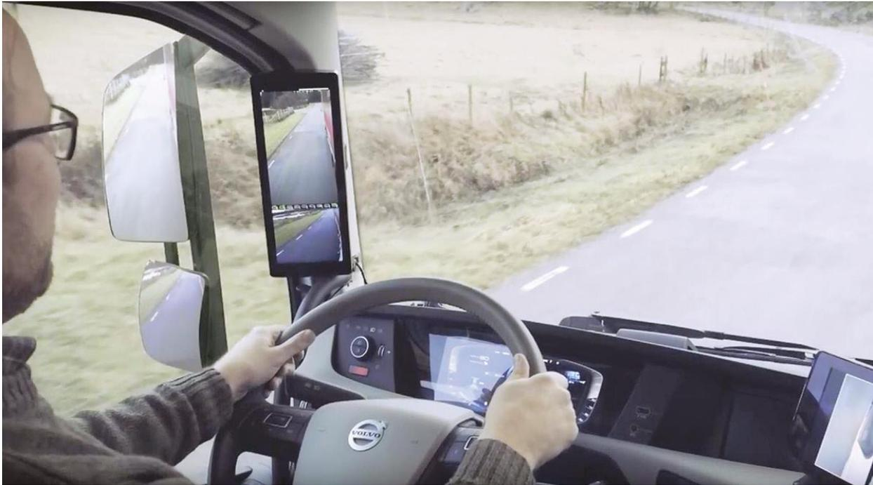
*A MirrorEye camera monitor system display inside a heavy-duty truck. (Orlaco Products)*
