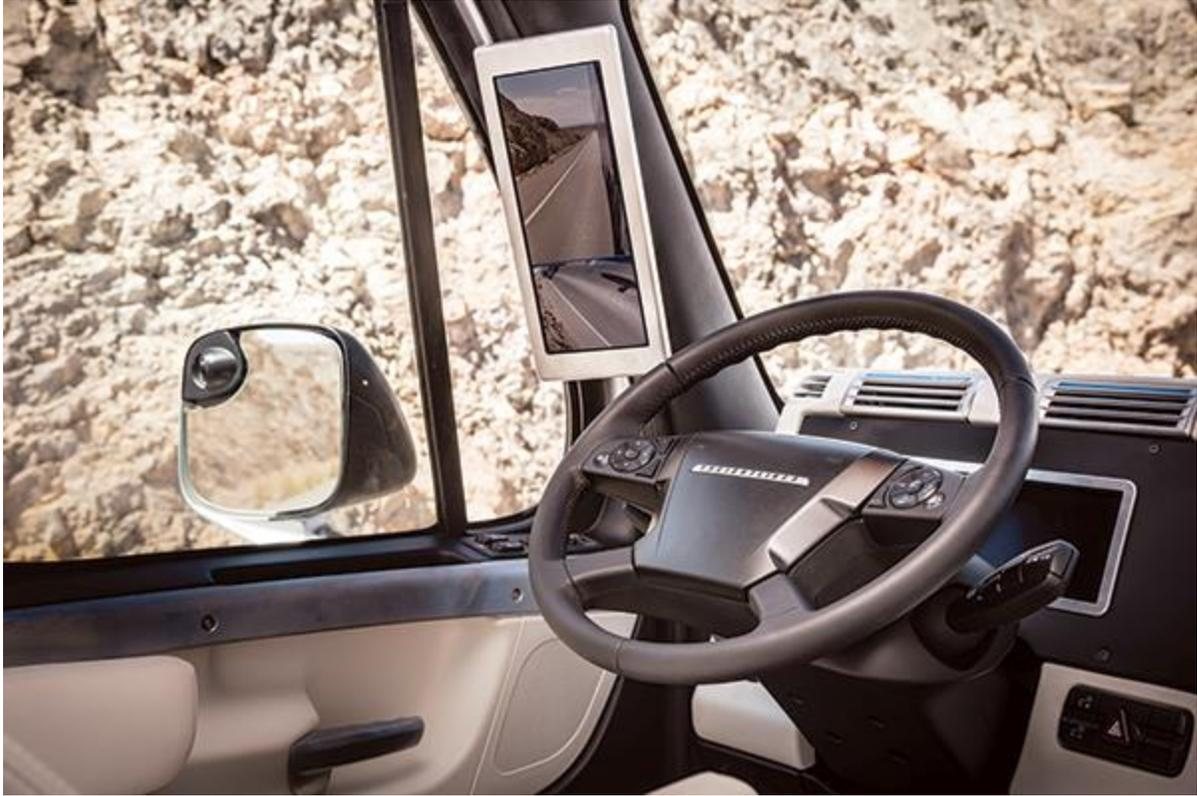
*A camera system in a Freightliner cab. (Daimler AG)*
