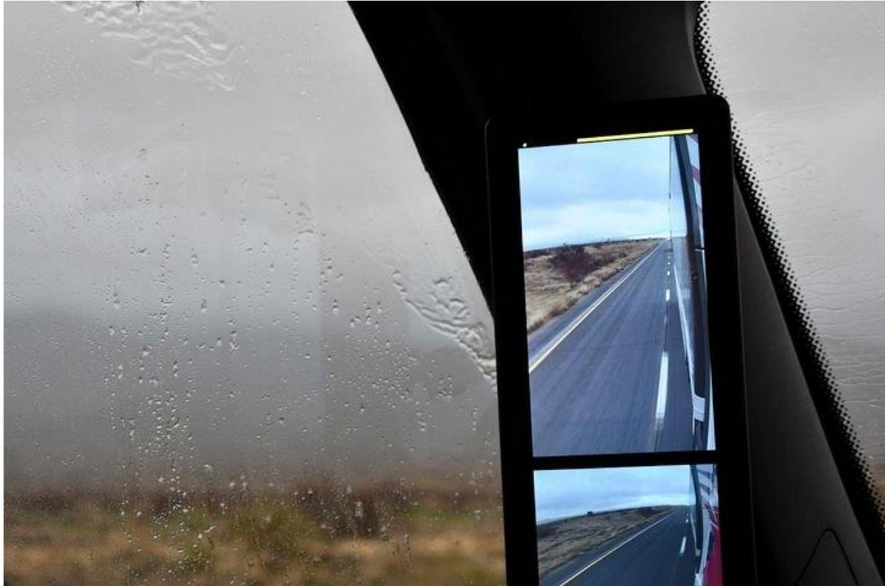
This supplied image shows how the camera lens remains clear while rain soaks the window, which would partially obscure visibility.
