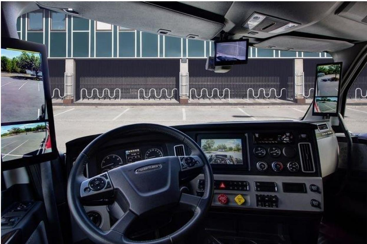
Taking into account a little distortion from the ultra-wide angle lens used to take this photo, the view from the driver's seat isn't much different with a monitor-based rear vision system.
