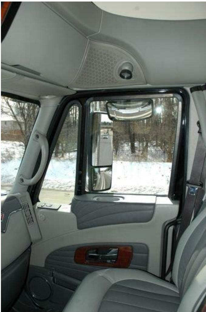
Compared to a more traditional arrangement, seen here, the monitor mounted to the A-pillar reduces the lateral blind spot created by the external mirror.
