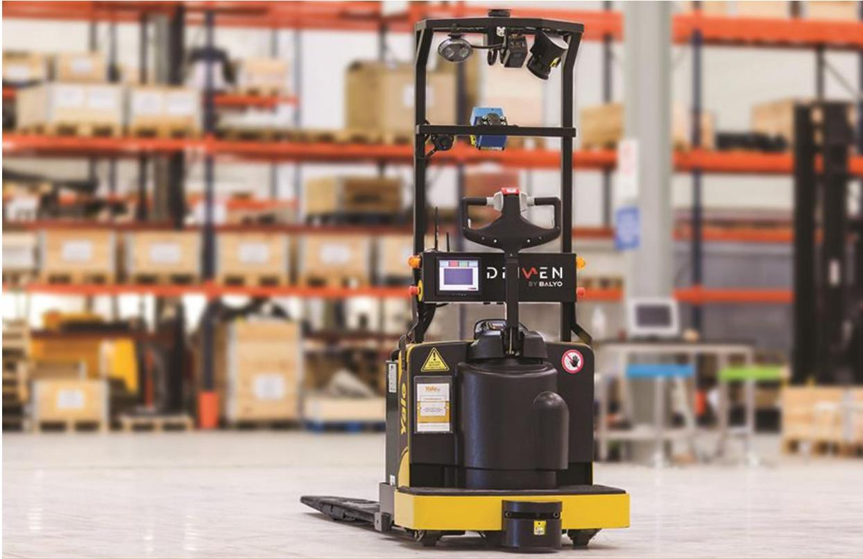
*Robotic end riders can automate workflows and moves that eat up considerable operator time with conventional vehicles.*
