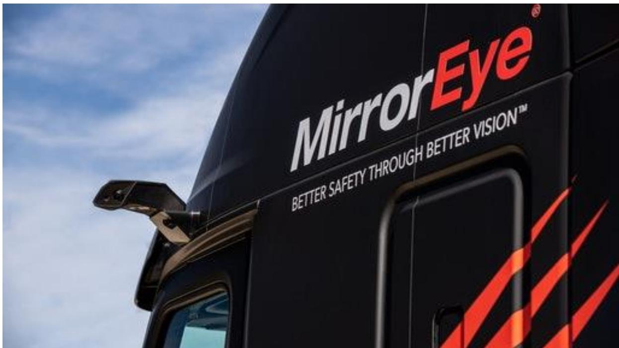
Tyson Foods, Inc. is testing a new technology to improve safety for its truck drivers. The Stoneridge MirrorEye Camera Monitor System (CMS) replaces traditional rear and side-view mirrors with integrated exterior mounted cameras and interior mounted monitors to help give drivers a more complete view of the road and the truck's surroundings, including common blind spots.
