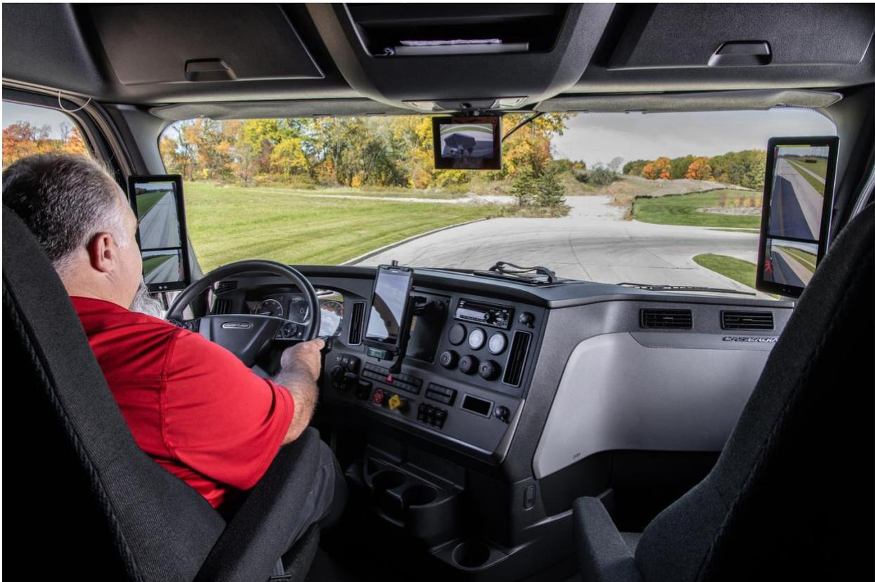
Tyson Foods, Inc. is testing a new technology to improve safety for its truck drivers. The Stoneridge MirrorEye Camera Monitor System (CMS) replaces traditional rear and side-view mirrors with integrated exterior mounted cameras and interior mounted monitors to help give
