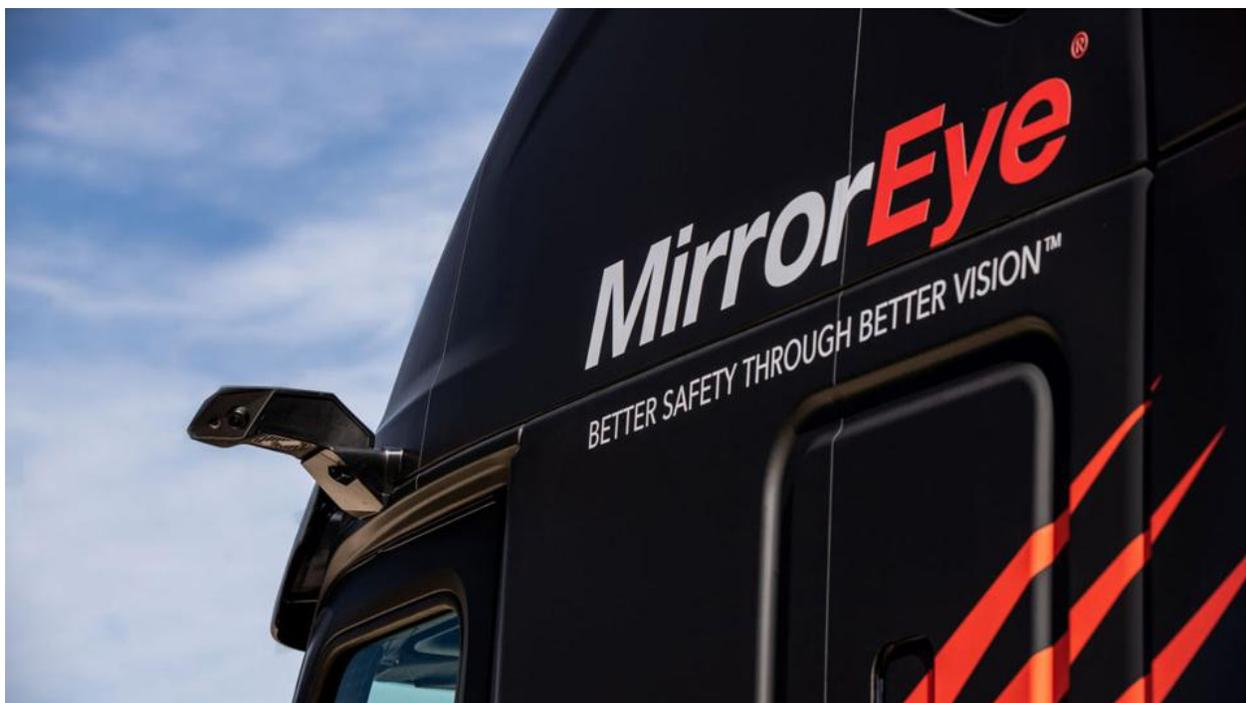
*Stoneridge's MirrorEye uses cameras to capture more of the road surrounding Class 8 commercial trucks than conventional side-mounted mirrors. Images are displayed on three interior monitors.*
